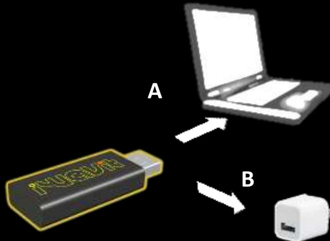
**Step 4. Option B:** Insert the USB dongle & IR Lightbar into any USB adaptor (sold separately). The dongle will now act like a **wireless IR Extender**. Use up to 16 in different rooms of your house if desired.
