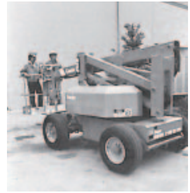
12-Boom retracted and lowered
