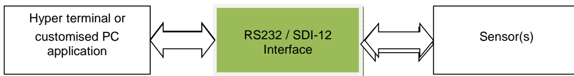
Figure 2 – TBS06 basic application setup
