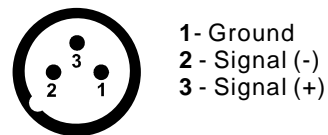
DMX-OUT XLR Connector - Socket:
