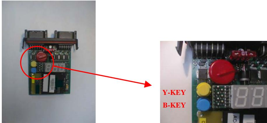
DBX-RX RECEIVER WITH TWO PUSHBUTTONS
