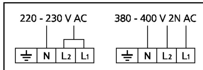
(this electrical connection lay-out is located near the power supply terminal board ). Tighten the cable gripper and re-fit the rear side-panel of the appliance.
