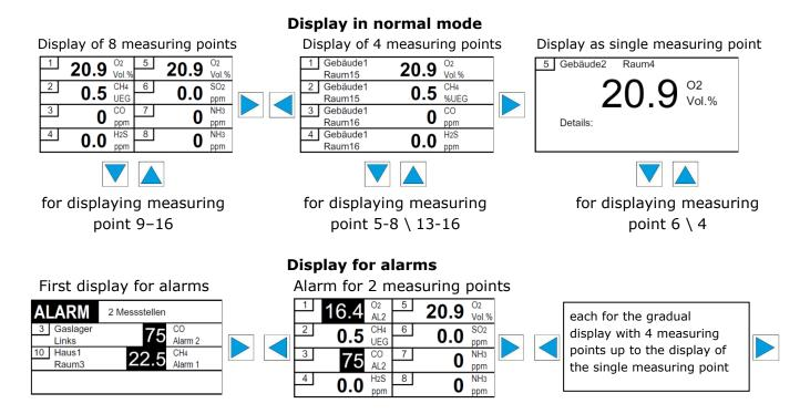
The display is backlit; the light intensity can be increased via any control button. In the event of a gas alarm or faults, the display lighting is automatically activated with a red background.
