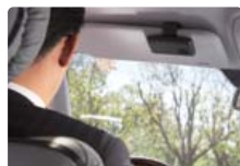
The Handsfree Kit must be placed in such a way that its buttons are facing the driver.
