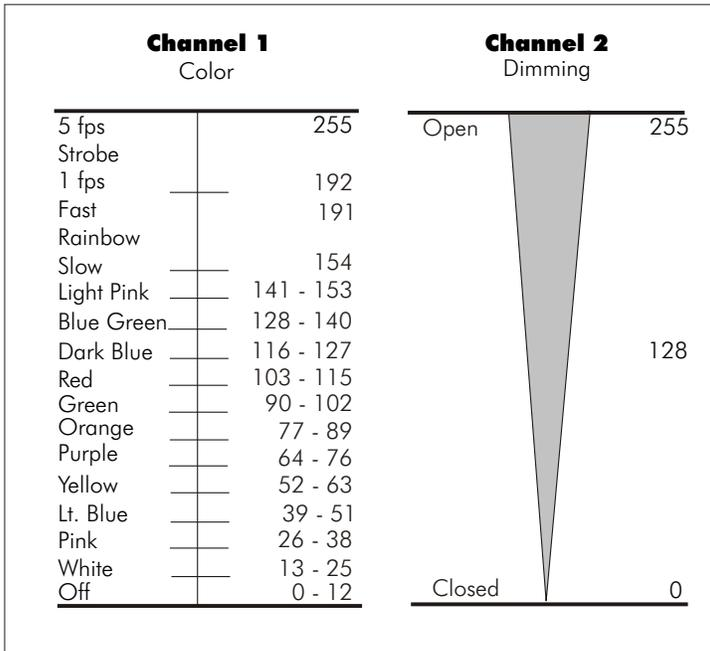
For example, when using a DMX512 controller on channel one, from position 103 to 115, a red-colored light will be projected. On channel two, at position 255, light output will be on full power.
