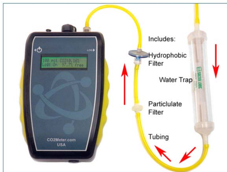
Figure 6: Filter Installation and Orientation
