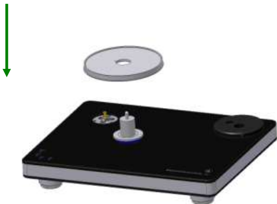
Pic. 6: Setting the sub-platter
