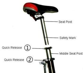
1-Before riding, you can loosen the quick release ②, adjust the saddle height up or down for your required fit, and then lock the quick release fastener ②. If the height is still not enough, please pull out the seat post to its correct height, then lock the quick-release fastener ①.
