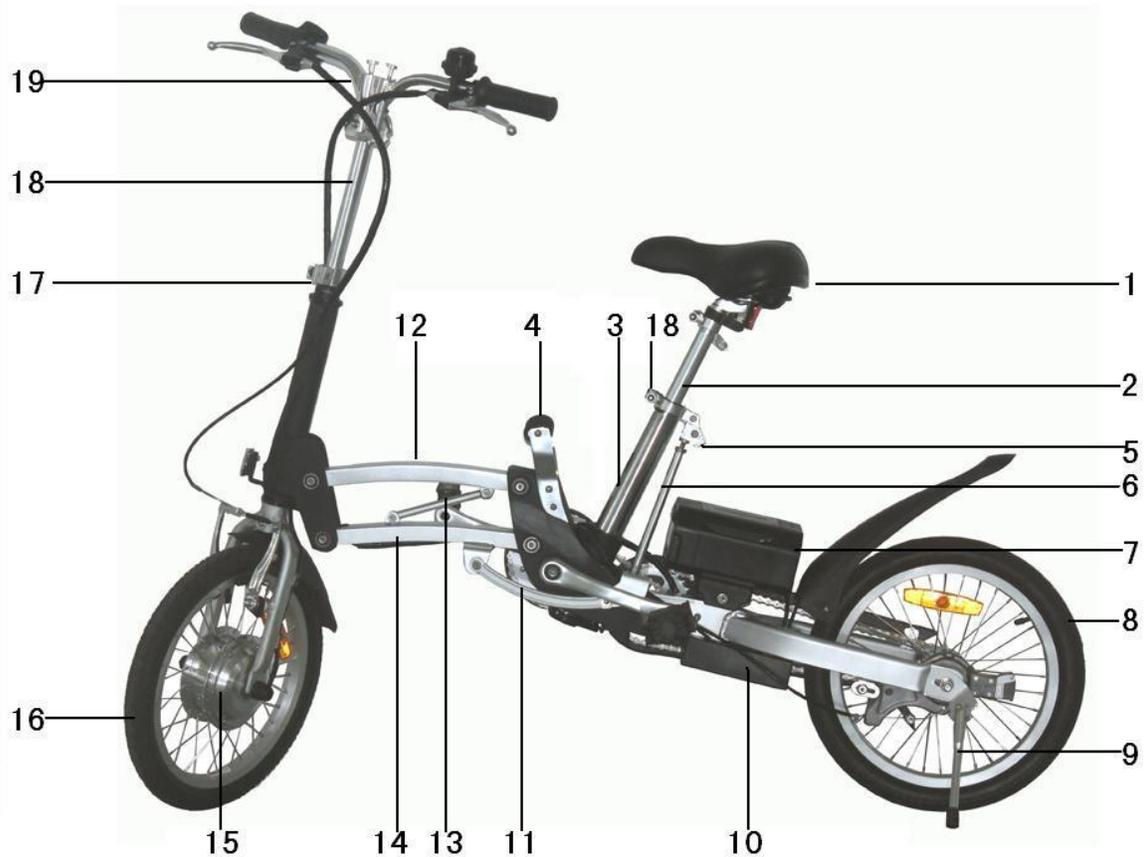
1: Saddle 2: Middle Seat Post 3: Big Seat Post 4: Folding Lift Handle 5: Lock System 6: Support Post 7: Li-ion Battery 8: Rear Wheel 9: Kickstand 10: Controller 11: Arc Link 12: Top Four-bar link 13: telescopic Link 14: Down Four-bar Link 15: DC Motor 16: Front Wheel 17: Quick-release 18: Stem 19: Foldable Handlebar
