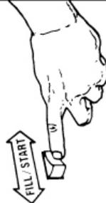
**10 PRESS PRIME SWITCHES TO PRIME CHEMICAL PUMPS AFTER REPLACING CHEMICAL CONTAINERS.**
