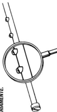
**4 IF SPRAY ARMS ARE CLOGGED, REMOVE BY TURNING BEARING CLOCKWISE.**
