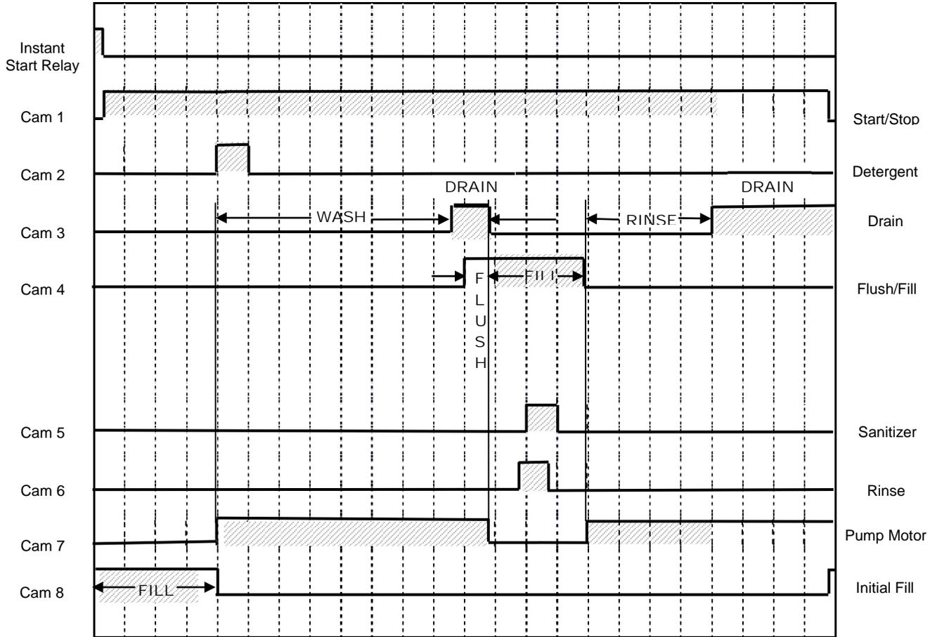
1. With the glasswasher powered up, toggling the START switch begins a cycle.
