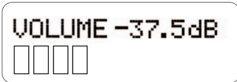
**Note:** dB values are a professional indication of the amplitude of an audio signal with full or maximum output achieved normally at 0dB. You will notice the LCD display on this amplifier will read minus dB figures up until zero which will indicate maximum output.
