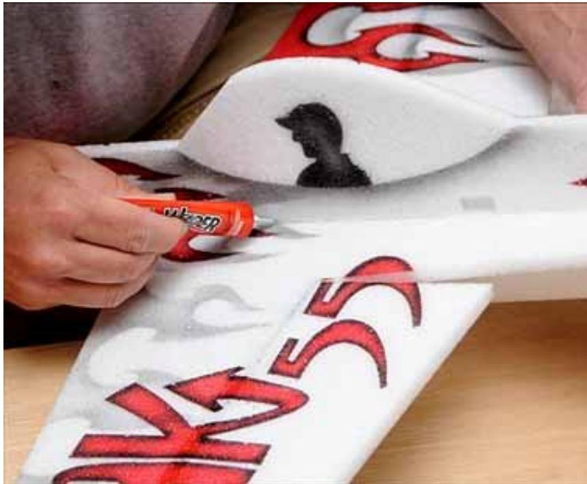
19. Test fit the plywood control horns in precut slots on top side of ailerons. Make sure the small hole in the control horn is directly above the hinge line. Once the fit has been verified remove the control horn and apply a small amount of Welders glue or super glue to the control horn and insert into slot in foam again making sure the hole in the control horn is directly above the hinge line.
