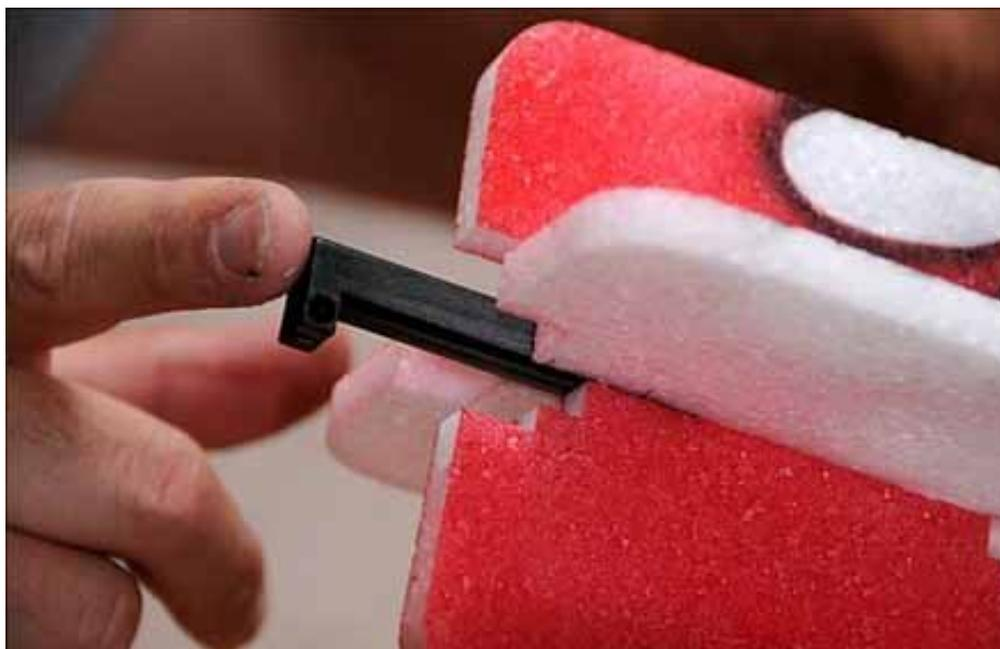
18. Put a bead of Welders glue on all sides of the upper & lower fuselage to wing assembly mating areas. Use a round dowel rod along the length of the joint form a nice fillet between fuselage and wing and tail assembly.
