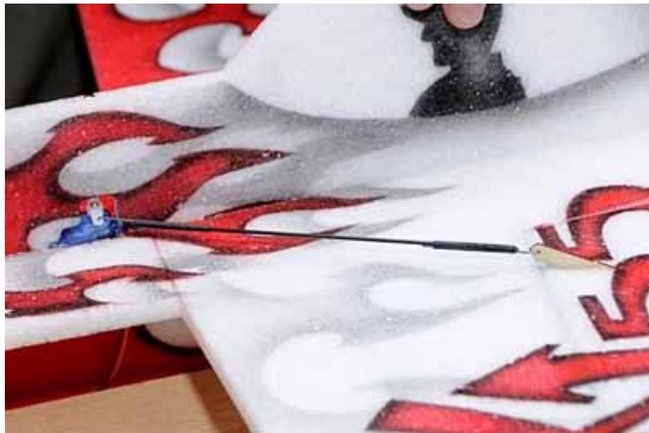
22. Install elevator servo in right side of fuselage and glue in place with hot glue.
