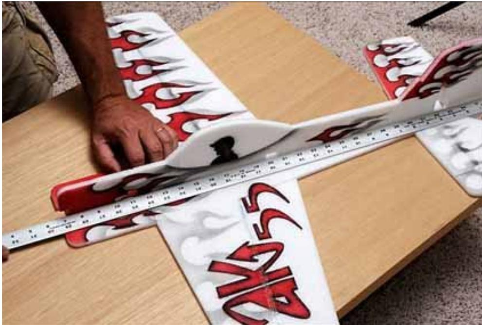
10. Next test fit the lower fuselage into the bottom side of wing and tail assembly. Make sure the lower fuselage and rudder fit flush against each other this joint will form the lower hinge.
