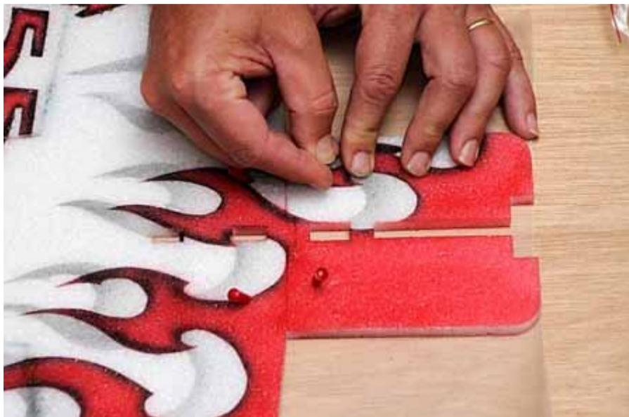
4. Repeat this process for the joints between the aft wing and forward side of aft horizontal fuselage assembly and between the aft side of the aft horizontal fuselage assembly and the forward side of the horizontal stabilizer and elevator assembly.
