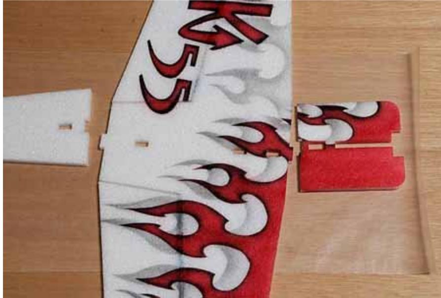
3. Starting at the front motor mount apply a small amount of Welders glue along the back edge of the motor mount and forward center section of the wing where the tab is located. Pin or weight parts down to hold them in place while the glue dries.
