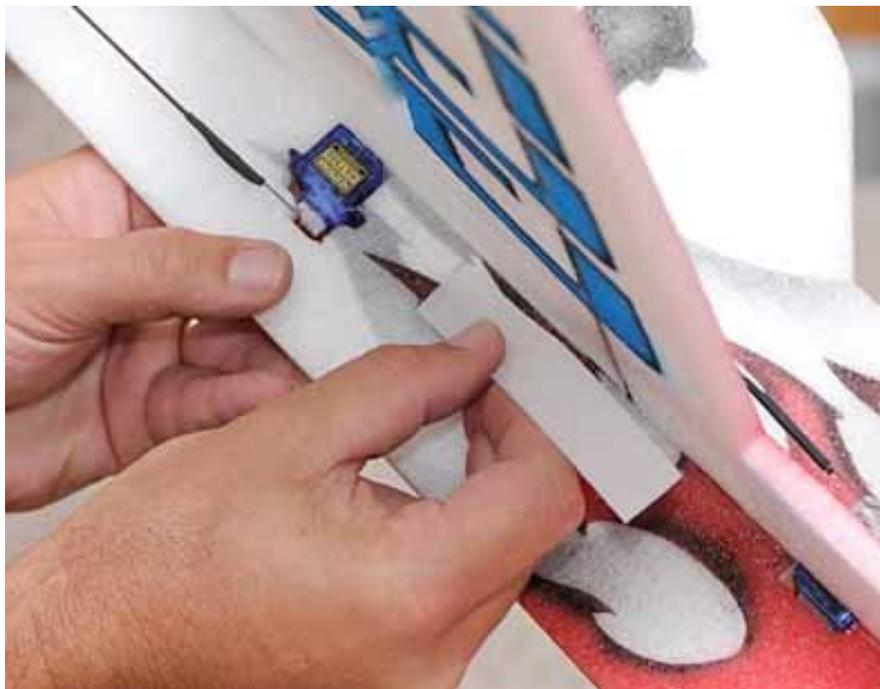
29. Put small piece of Velcro on left side for esc & receiver again we use the ruff side on the plane and the fuzzy side on the esc and receiver.
