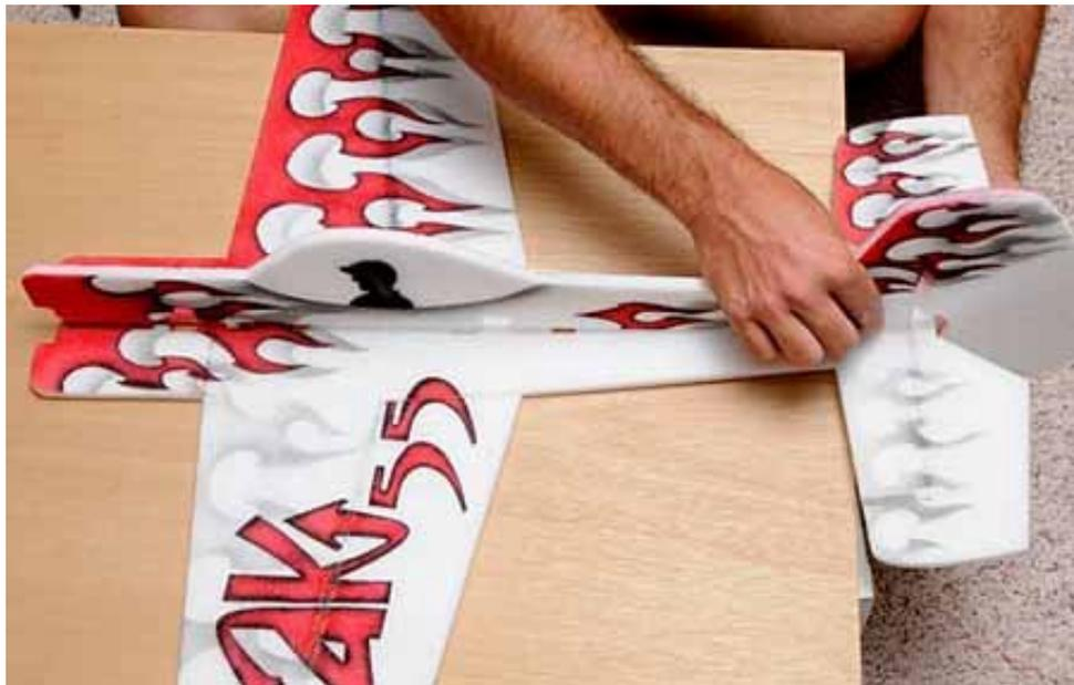
7. Once alignment is verified glue top of fuselage to top of wing assembly. Use a thin bead of Welders glue on the lower mating surface of the upper fuselage spreading glue evenly with your finger. Do not put glue in the area forward of the aileron servo cutout or forward where the motor mount will go.
