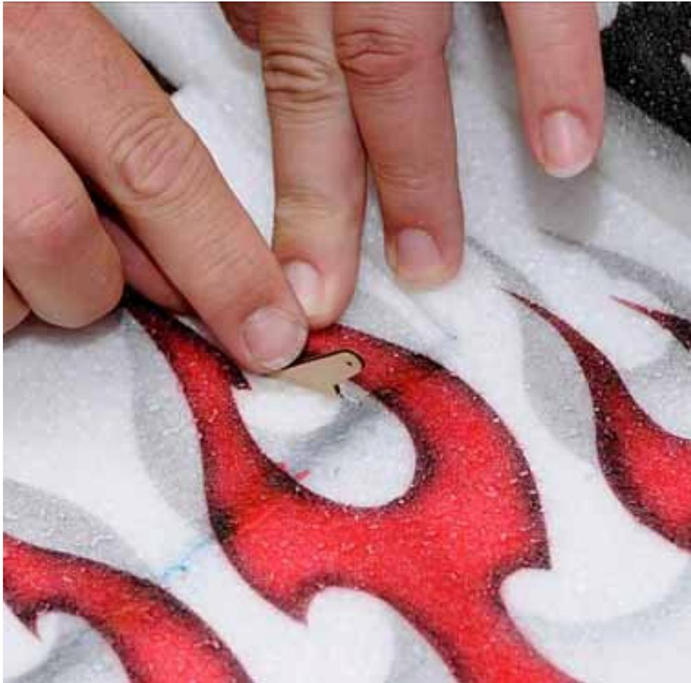
20. Install the pre-made end of the aileron control horn into the plywood control horn that was just glued into the aileron control surface.
