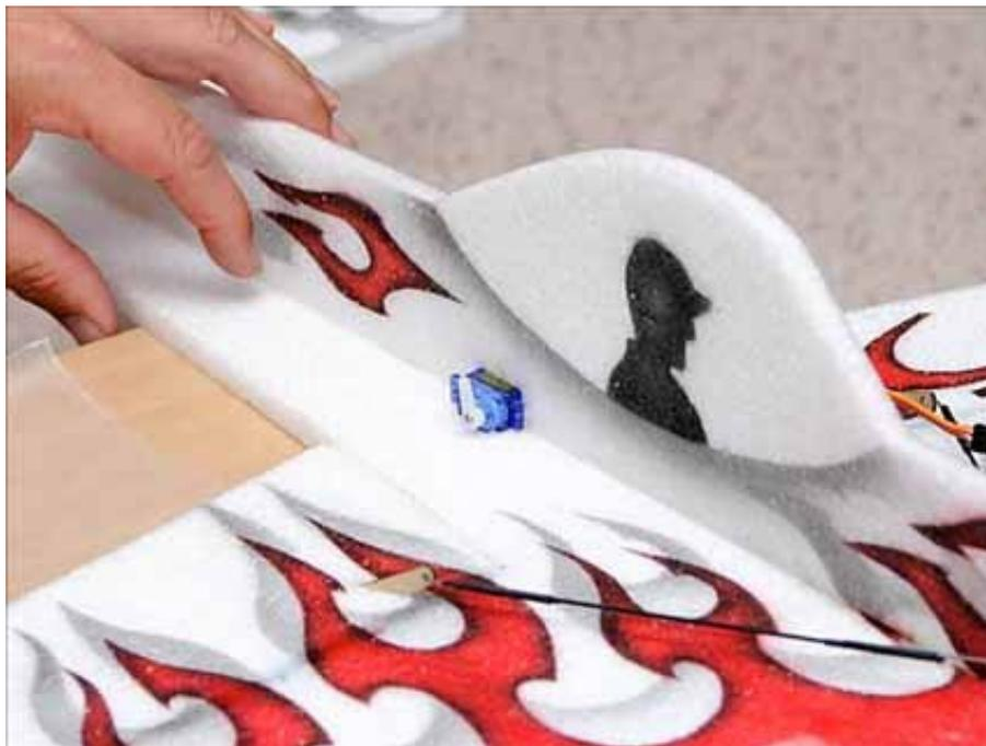
23. Cut a small slot in foam for servo wires to feed thru to receiver as show in picture.
