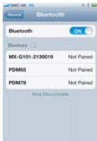
2.6 Enter password “8888” and press “Pair” button (it will be paired automatically if device is paired before).
