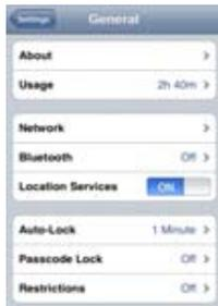
2.5 Turn the Bluetooth on and select the serial no of your 3BaysGSA Device from the list of Devices (serial no can be found on your device and packaging)
