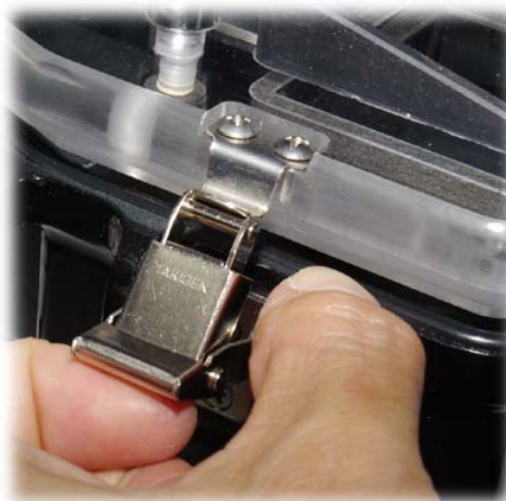
Lift Tab at End of Lever to Push the Hook and Lid Up
