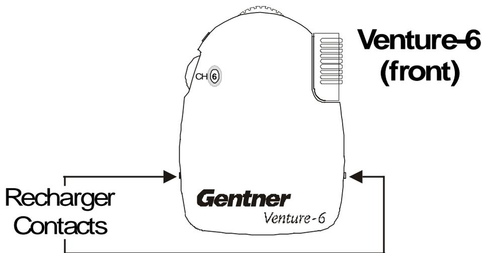
These contacts may be used in conjunction with Gentner's BC-10A for quick and easy recharging. Simply place the Venture-6 receiver in the BC-10A charger when not in use and it will automatically recharge for the next usage.
